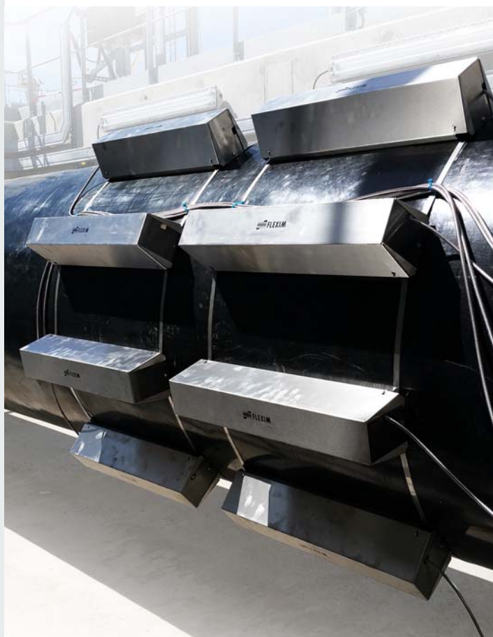
4 transducer pairs at one measuring point
